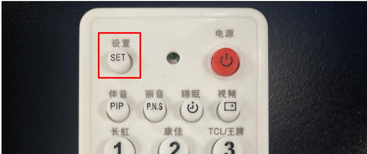
Figure 12 - The universal remote includes a function for searching for the correct commands
