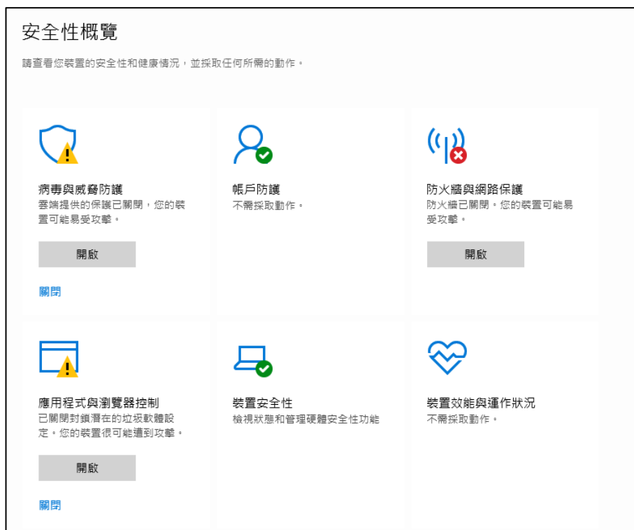
Figure 17 - Windows Firewall is disabled in A1 Signage
